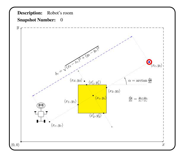
position  $\langle x_r + \delta_r \cos \alpha, y_r + \delta_r \sin \alpha \rangle$ . Therefore, the robot *always* moves using the method (in C++ syntax):
