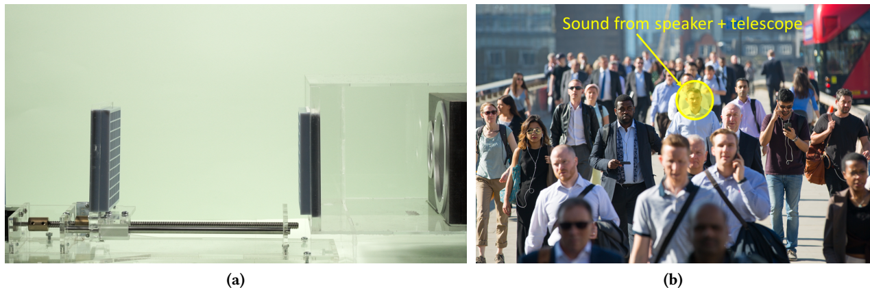
Figure 8: Acoustic telescope configuration, using two converging lenses of the same focal length: (a) side view and (b) a potential application, connecting acoustically with a single person in a crowd. Front view in Figure 1.
